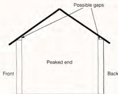
In this view exaggerating the thickness of the walls of a gable-ended structure, note the gaps which result at the tops of the side walls if the sides overlap the peaked ends. To avoid this problem, have the peaked ends overlap and cover the sides.
