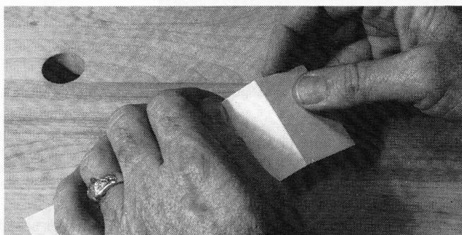
When cutting styrene with a square, hold the base of the square over the edge of the workbench or cutting board. Use your thumb to hold the blade tightly on the sheet and support the square with your index finger. Score the sheet, then snap it off.
