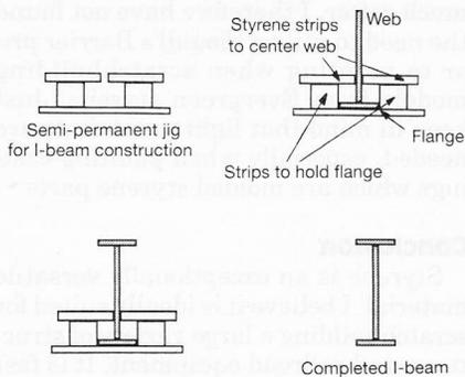
A semi-permanent jig for producing I-beams may be constructed from strip styrene. The web is assembled to the first flange, then the piece is inverted to add the second one.
