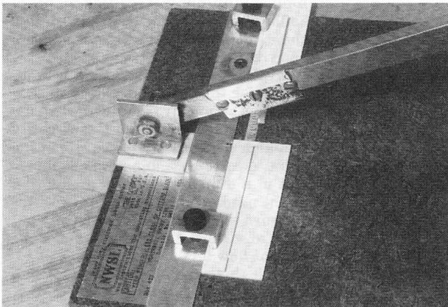
The tools needed for laying out the work are common ones: scale rulers, squares, draftsman's dividers and dial calipers. The NorthWest Short Line Chopper is an indispensable tool for cutting strips to length. To offset a worn hardboard base, place a piece of .040"
