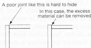
Watch joint alignment at corners. Note that it is much easier to correct alignment problems if an edge overlaps a side, rather than vice-versa.
