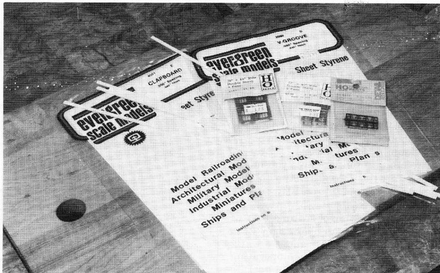
The materials for building with styrene include styrene sheet in several thicknesses, strip styrene (it comes in both dimensional and scale sizes) and styrene detail parts.
