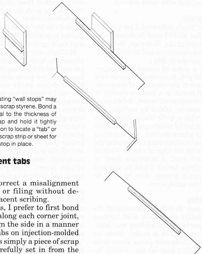
The tab will insure that the adjacent wall is correctly located in relation to the edge.
