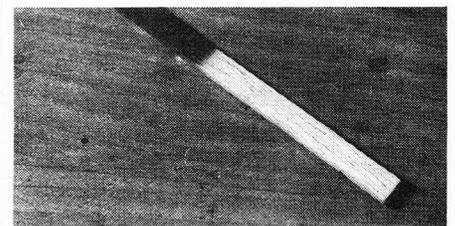
When desired, wood grain effects on styrene sheet or strip may be done with coarse sandpaper or a metal-bristled brush.
