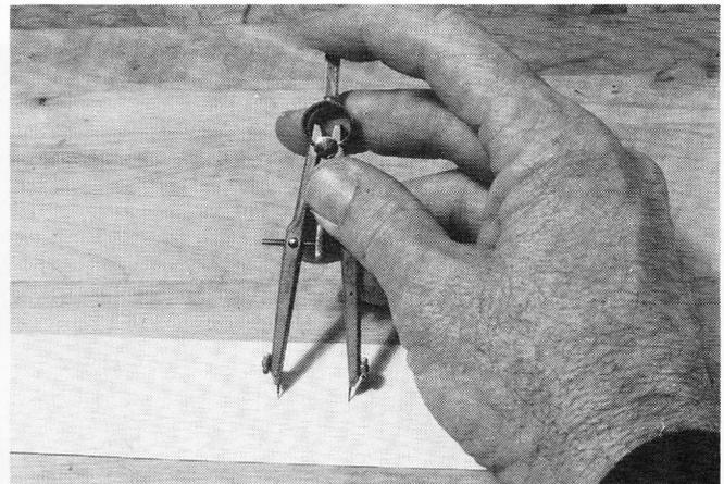
sheet under the cutting area. A .040" shim must be used under the cutting arm hinge to keep it parallel. Note the new fence. Draftsman's dividers may be used to "walk off" dimensions; circle the points with a pencil.
