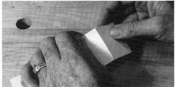
When cutting styrene with a square, hold the base of the square over the edge of the workbench or cutting board. Use your thumb to hold the blade tightly on the sheet and support the square with your index finger. Score the sheet, then snap it off.
