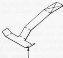
The width of the slider portion must be wide enough to maintain rail contact but not too wide to short out at the switches.
