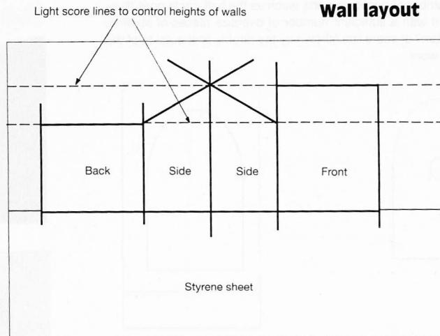
Layout of a typical "lean-to" structure. First score a line to become the bottom of the four sides; then lightly score guide lines for the height of the front and the back. Using dividers, set the width of the two sides; reset the dividers and mark the width of the front and back. Now deepen the appropriate score lines and snap the parts apart.
