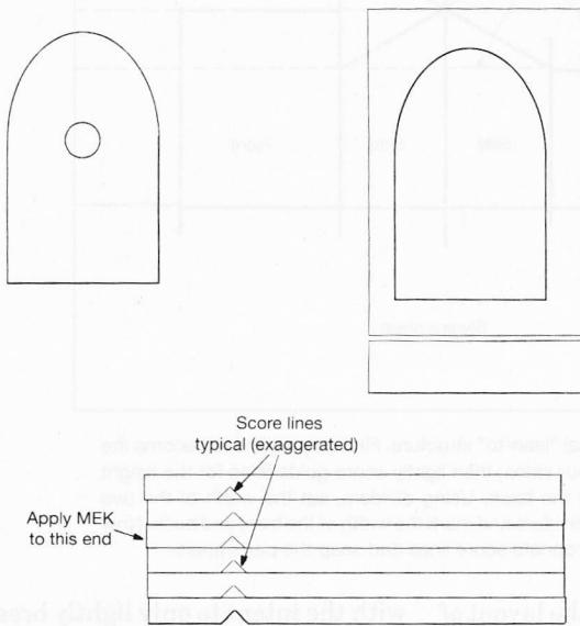
Stack the pieces together and apply MEK to the joints on the "waste" end of the stack as shown. The score lines will prevent the MEK from flowing through the layers to the opposite end of the stack. File the stack to the desired shape and cut apart.
