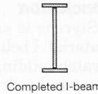
A semi-permanent jig for producing I-beams may be constructed from strip styrene. The web is assembled to the first flange, then the piece is inverted to add the second one.
