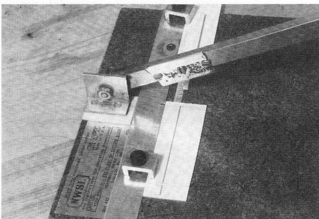
The tools needed for laying out the work are common ones: scale rules, squares, draftsman's dividers and dial calipers. The North-West Short Line Chopper is an indispensable tool for cutting strips to length. To offset a worn hardboard base, place a piece of .040"
