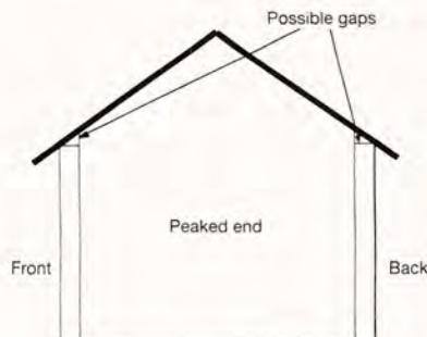
In this view exaggerating the thickness of the walls of a gable-ended structure, note the gaps which result at the tops of the side walls if the sides overlap the peaked ends. To avoid this problem, have the peaked ends overlap and cover the sides.
