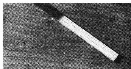
When desired, wood grain effects on styrene sheet or strip may be done with coarse sandpaper or a metal-bristled brush.
