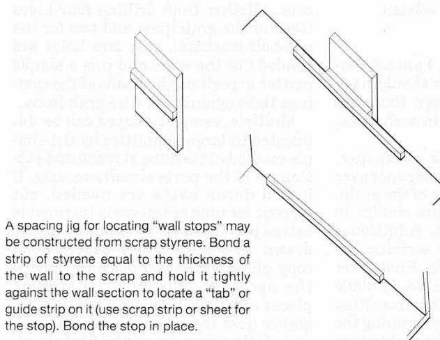
A spacing jig for locating "wall stops" may be constructed from scrap styrene. Bond a strip of styrene equal to the thickness of the wall to the scrap and hold it tightly against the wall section to locate a "tab" or guide strip on it (use scrap strip or sheet for the stop). Bond the stop in place.
