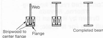
For a temporary jig to make I-beams or channel, stripwood of the appropriate width is used to center the web on the flange. After gluing the first flange in place, turn the assembly over and attach the second flange in a like manner.
