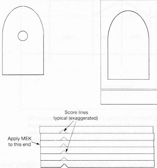
Stack the pieces together and apply MEK to the joints on the "waste" end of the stack as shown. The score lines will prevent the MEK from flowing through the layers to the opposite end of the stack. File the stack to the desired shape and cut apart.
