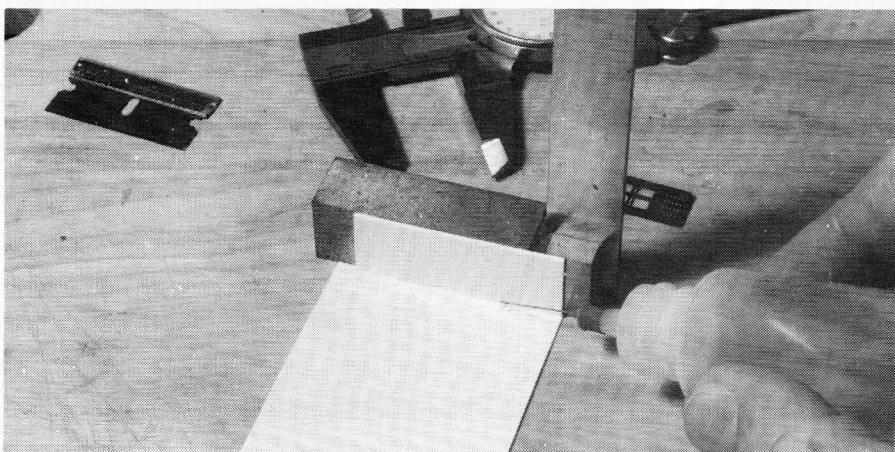
MEK or other solvent-type styrene cements are best applied with an A-West needlepoint applicator. A machinist's square will insure that assemblies are square when being glued.
