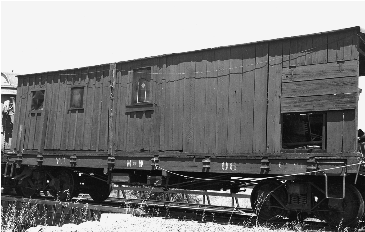
M of W 06 reveals its obvious ancestry as a flat car in this photo of the car in the Merced yards. - Bill Pennington photo, author's collection
