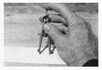
sheet under the cutting area. A .040" shim must be used under the cutting arm hinge to keep it parallel. Note the new fence. Draftsman's dividers may be used to "walk off" dimensions; circle the points with a pencil.
