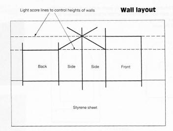
Layout of a typical "lean-to" structure. First score a line to become the bottom of the four sides; then lightly score guide lines for the height of the front and the back. Using dividers, set the width of the two sides; reset the dividers and mark the width of the front and back. Now deepen the appropriate score lines and snap the parts apart.
