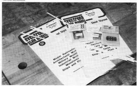
The materials for building with styrene include styrene sheet in several thicknesses, strip styrene (it comes in both dimensional and scale sizes) and styrene detail parts.
