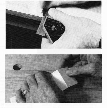
When cutting styrene with a square, hold the base of the square over the edge of the workbench or cutting board. Use your thumb to hold the blade tightly on the sheet and support the square with your index finger. Score the sheet, then snap it off.
