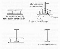
A semi-permanent jig for producing lbeams may be constructed from strip styrene. The web is assembled to the first flange, then the piece is inverted to add the second one.
