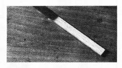
When desired, wood grain effects on styrene sheet or strip may be done with coarse sandpaper or a metail-bristled brush.
