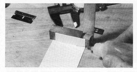
MEK or other solvent-type styrene cements are best applied with an A-West needlepoint applicator. A machinist's square will insure that assemblies are square when being glued.
