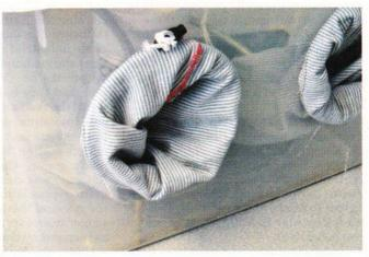
clips to hold the lid closed. The sleeves (above right) are from an old long sleeve shirt. They are hemmed and fit over plywood rings and secured with elastic cord to lock them in place.
