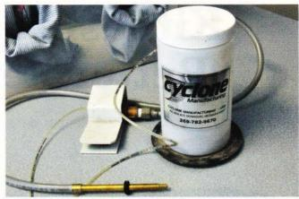
(above right) are the shop vacuum connection, a pencil sandblaster, a container of abrasive and a foot pedal air valve.
