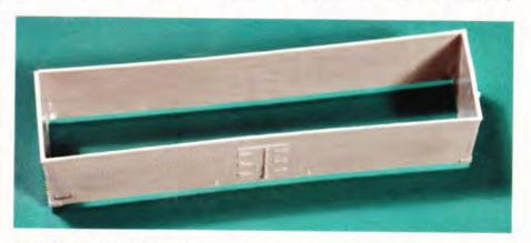
The sides and ends of this refrigerator car kit (above) have been glued together. Although the sides of resin kits can sometimes be slightly warped, the sides on this refrigerator car are just flexible because they are thin. The basic carbody (below) is seen with a pair of floor spacers clamped in place. The body is right side up with the floor below it.
