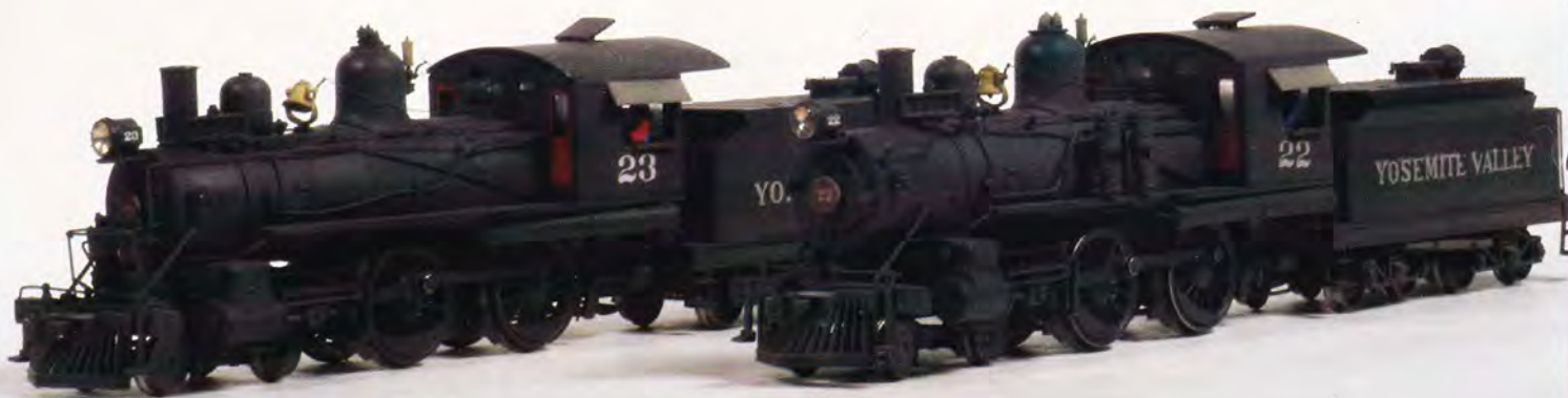
Fig. 7 Finished models. Here we see completed YV 4-4-0s nos. 23 and 22. In this view, you can see some of the detail differences between these two locomotives, such as the location of the air compressors.
